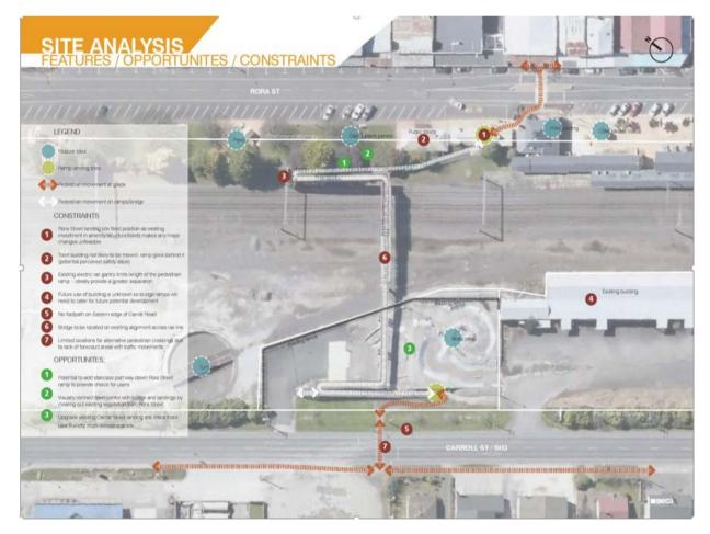
Fig.3: Site layout and constraints
